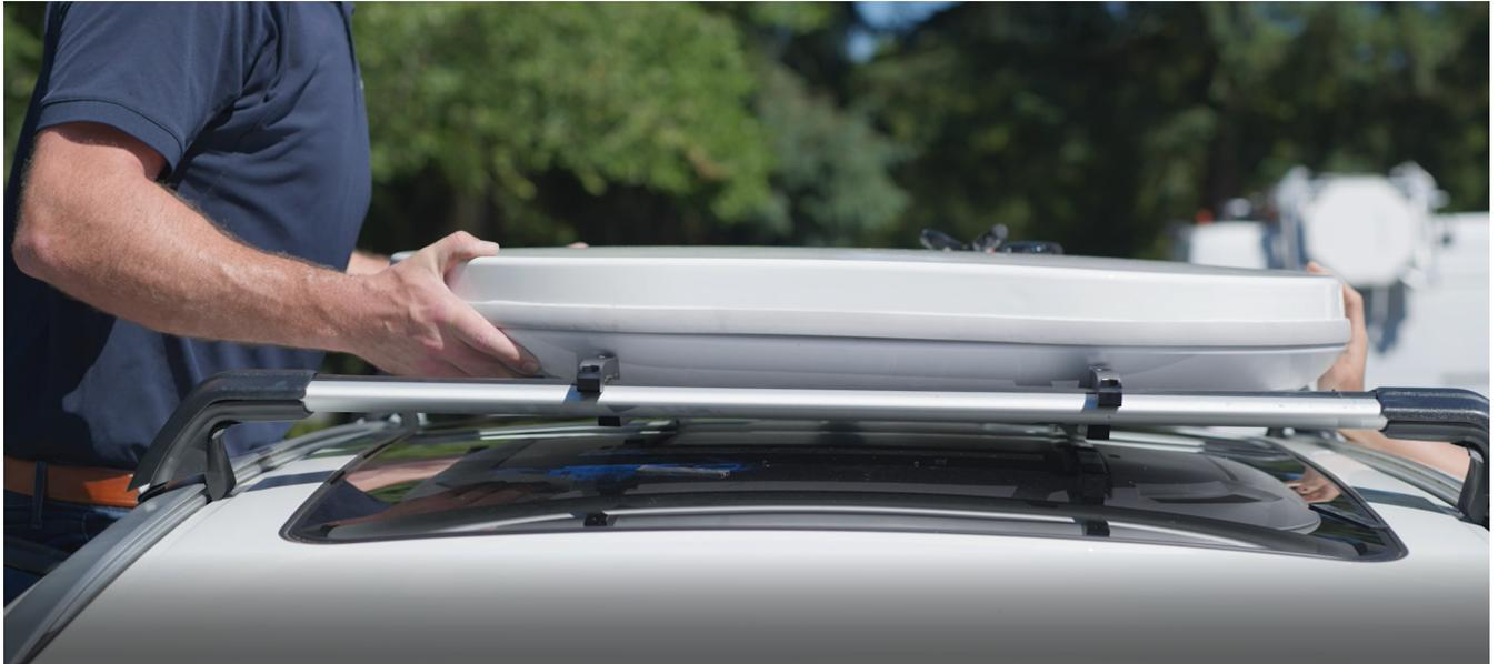
3. Ensure the rail/antenna assembly is roughly centered on laterally on the cross bars. Once roof rack is in desired lateral location, remove the tear off cardboard pads individually.
