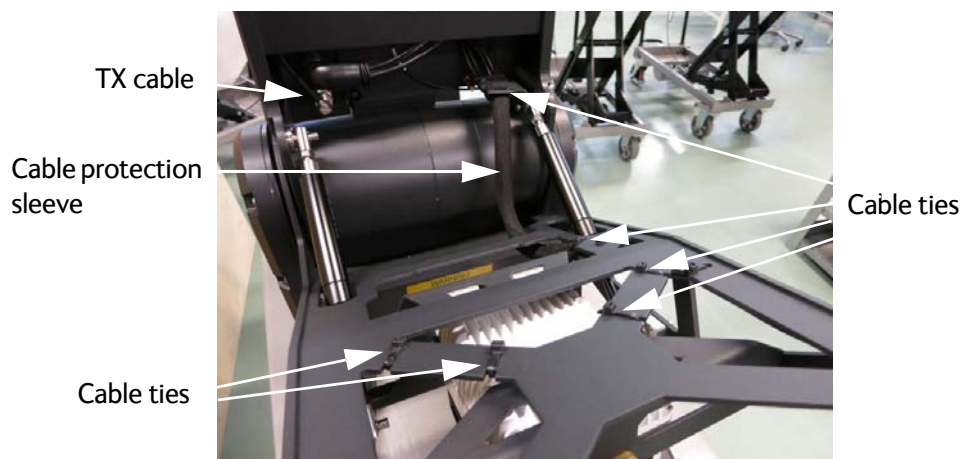
Figure 7-18: BUC installation, TX cable
