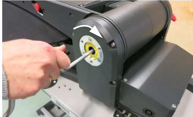
Figure 7-8: Manual elevation adjustment
